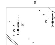
FIXAR CAVILHAS NAS FURAÇÕES LATERAIS E POSICIONAR O TAMBOR MINIFIX FIXAR BUCHAS DE NYLON NAS LATERAIS COM AUXÍLIO DE UM MARTELO DE BORRACHA
