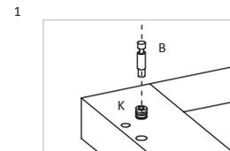
FIXAR BUCHAS DE NYLON NO TAMPO COM AUXÍLIO DO MARTELO DE BORRACHA E PARAFUSAR CHAPA TRAVA ARMARIO NO TAMPO EM SUAS RESPECTIVAS MARCAÇÕES
